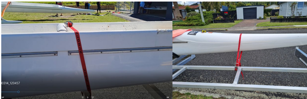
Figure 1 - Ratchet position at Taumanu - Ratchet over top of hull opening, avoid ratchet against hull surface.
